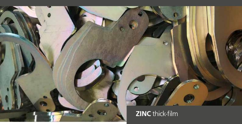
One of the most frequently used processes to achieve secure and cost-effective protection against corrosion is the electroplating of zinc. Steel workpieces whose surfaces are galvanized offer effective corrosion protection. Zinc has a negative potential compared to iron. Zinc is therefore very well suited as a sacrificial anode for the cathodic corrosion protection of iron alloys (remote protective action).
